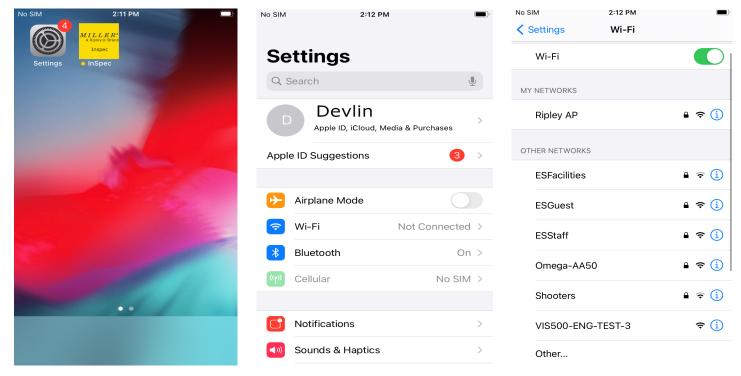
Next wait until a SSID Showing "VIS500" followed by the 4 digit start to your serial number. Once that appears click it and wait for the check mark to appear next to the ssid. Finally open or return to the Mobile InSpec application.
