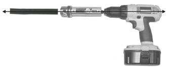
**4.** To ensure consistent and accurate removal of covering, the cable must be as straight as possible. **Slide the tool onto the cable until the cable end is up against the stripping blade.** Ensure that the tool is aligned properly with the cable axis.
