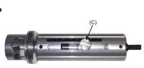
**2.** Set the strip length. Loosen the thumb knob, slide the stop to align the red band to the desired strip length, and re-tighten.
