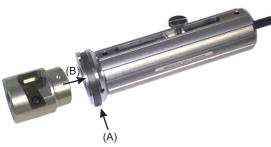
**1.** Insert bushing into tool. Depress the lock collar at the front of the tool, insert the bushing, and rotate it to snap it in place.
