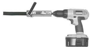
5. Operate the drill at low speed and apply slight forward pressure to the tool. The cable covering will be removed until the conductor reaches the internal stop. The blade will automatically sever the covering evenly at the end of the cut. Stop the drill when the cut has ended and avoid freewheeling. Remove the tool from the cable.Do not remove the tool while the drill is turning.
