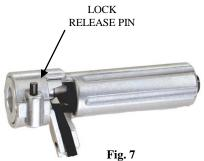
(Fig. 7) To remove the bushing, depress the lock release pin on the housing and slide the bushing out.
