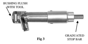
**Step 3.** (Fig. 3) To adjust the stop bar for desired length of conductor exposure, loosen set screw located on the underside of the graduated stop bar on the tool body. Adjust the stop bar to the desired length of exposed conductor needed and tighten the set screw.
