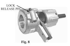
(Fig. 8) To remove the bushing, depress the lock release pin on the housing and slide the bushing out.
