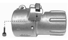
Fig. 9 - Blade Locking Screw
