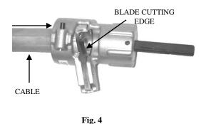
**Step 4.** (Fig. 4) To strip the insulation, insert the cable into the WS6-M until it comes in contact with cutting edge of the blade. Always check the blade position with respect to the conductor, before stripping the insulation.
