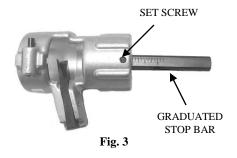
**Step 3.** (Fig. 3) To adjust the stop bar for desired length of conductor exposure, loosen set screw located on the end of the tool body directly above the stop bar. Adjust the stop bar to the desired length of insulation to be stripped and tighten the set screw.
