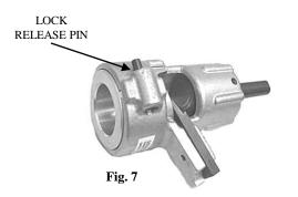
(Fig. 7) To remove the bushing, depress the lock release pin on the housing and slide the bushing out.
