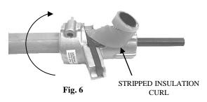
**Step 6.** (Fig. 6) Rotate the tool clockwise around the cable to remove the insulation. Insulation will peel off until the cable conductor reaches the stop bar. The blade will automatically sever the insulation cleanly at the end of the cut.
