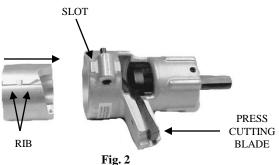
**Step 2.** (Fig. 2) To insert the bushing into the WS6-M, line up rib on the bushing with the slot on the WS6-M housing. Raise the cutting blade by depressing outer end and insert the bushing until it locks into place.
