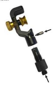
**4.** Test the blade adjustment: index the blade to full depth, then back off to zero depth.
